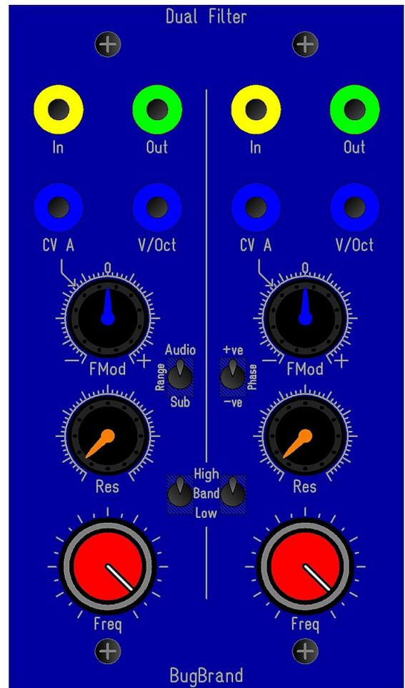
The Sub mode on the left-hand section switches in extra filter capacitors to shift the range into sub-audio frequencies.
