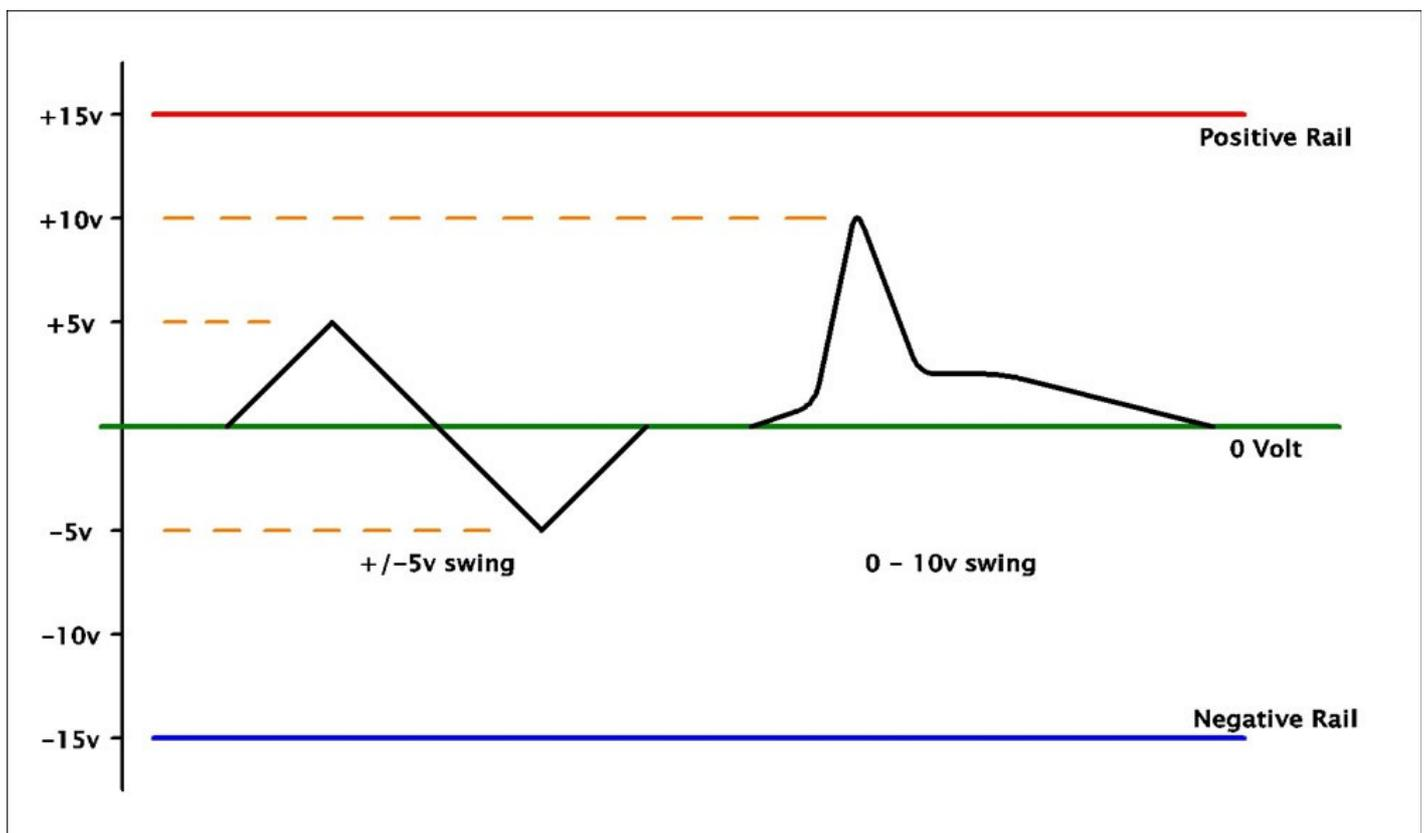
Of course, there can be slight exceptions to note – signals coming from a VCA may well be less than 10V P-to-P (unless the VCA is 'fully open'), adding resonance via the Filters can increase amplitude and mixing several full-scale signals together can result in larger total swings. But you always have plenty of headroom before 'hitting the rails' (as signals can never exceed the bounds of the system power).
