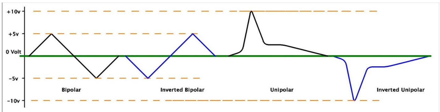
It is important to consider the waveform's behaviour when applying it as a modulation signal. The modulation voltage (after input attenuverter) is summed with the value set by the main control dial, with positive voltages adding to the main sum and negative voltages subtracting. As such:
