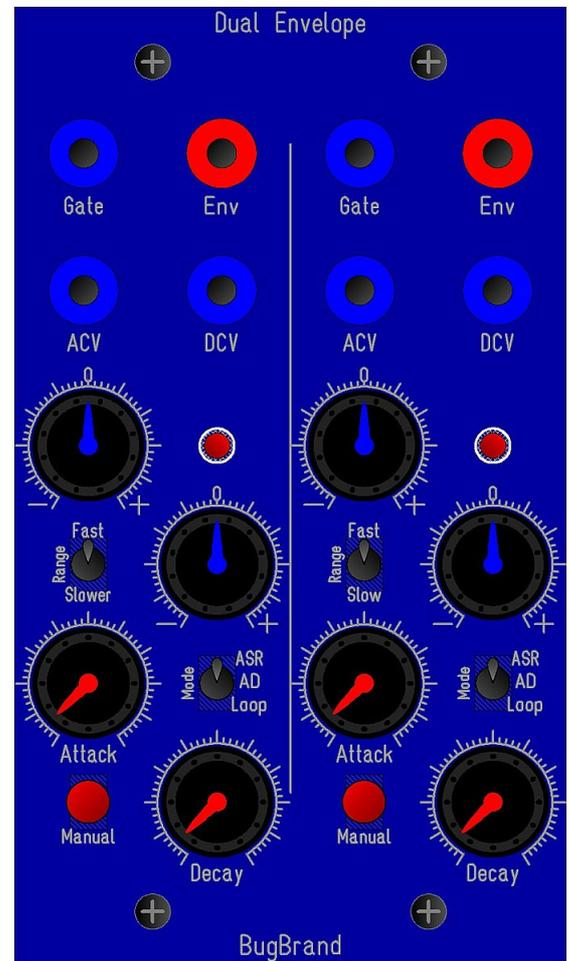
The Fast range offers audio rates, primarily for use in Loop mode, while the Slow(er) range offers sub-audio rates for more typical Envelope usage. Note that faster Attack/Decay rates are achieved by turning the dials clockwise – this may seem counter-intuitive, but makes more sense if thinking of it raising the frequency of an oscillator.
