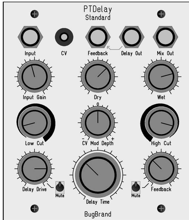
The **BugBrand PT Delay Standard** is built around the Princeton Technology PT2399 Digital Delay chip. While the PT2399 itself allows easy implementation of basic delay effects, it only really shines when wrapped up in supporting blanket of analogue circuitry. [Though, of course, once the chip feels safe & happy we start to abuse it, underclocking it so that it spits digital chatter.] Evolving over several years, the PT Delay has become a supremely characterful and tactile delay processor.
