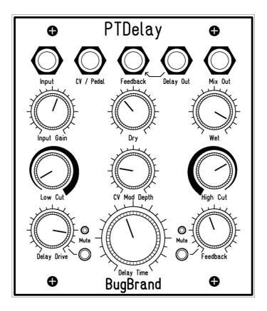
The **BugBrand PT Delay Standard** is centred around a Digital Delay chip, the Princeton Technology PT2399. While the chip is digital, its design approaches are already quite analogue and around this core is added highly specific analogue circuitry to create a characterful and tactile delay processor.
