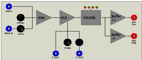
are DC coupled and this is notable both for the fact that LFO waveforms can be processed and that applying DC offsets can really alter the resulting waves. A DC offset can either be applied with the Offset dial (centre equals zero offset) or I will typically apply an LFO to the 2nd input and use the level control to dial in a little of this - the result sounds somewhat similar to pulse-width modulation. (eg. Try this with DC generated from the CTL2 Joystick)
