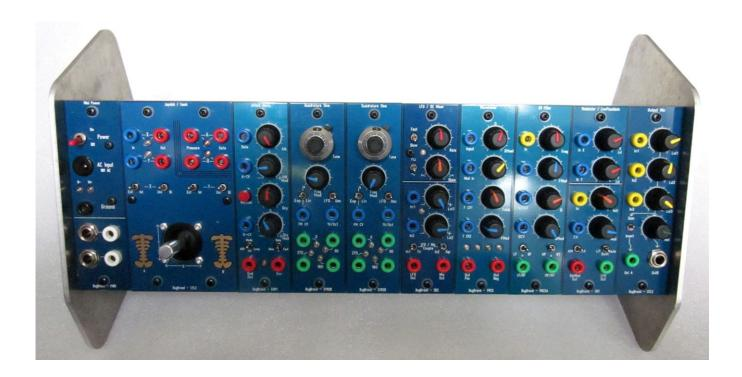
The 1Frame SynthVoice arrangement presents a combination of modules aiming roughly along the lines of traditional subtractive synthesis (VCO  $\rightarrow$  VCF  $\rightarrow$  VCA). The patchable, modular approach not only gives great scope and versatility around such areas, but also opens up many more esoteric arenas for exploration.
